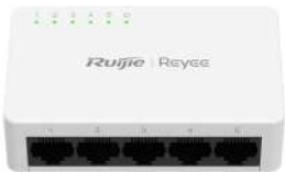
RG-ES05F 5-port 10/100 Mbps unmanaged non-PoE switch
