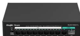
RG-ES110GS-P-L 10-port 10/100/1000 Mbps unmanaged PoE switch
