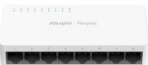
RG-ES08G-L 8-port 10/100/1000 Mbps unmanaged non-PoE switch
